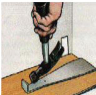
The last board of a run can be tapped into place with a pulling iron and a hammer or mallet.
